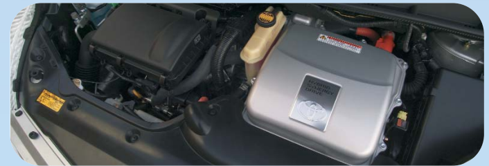
Under the hood—a 1.5 liter gas engine (left) and power inverter (right)
